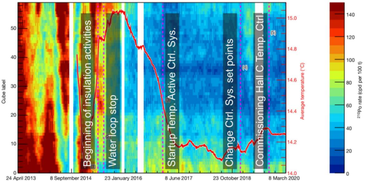
Stabilization measures have been extremely effective in reducing  $^{210}\text{Po}$  motions
