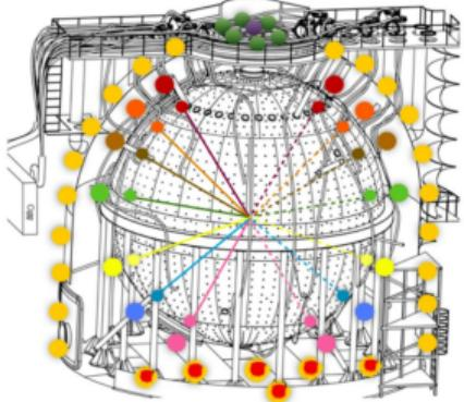
Latitudinal Temperature Probe System
