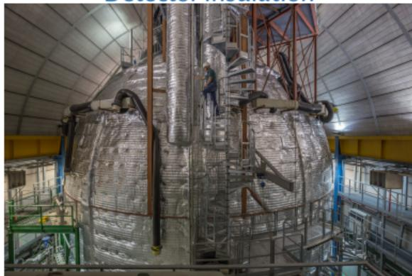
Thermal Insulation System (TIS) Double layer of mineral wool (20 cm)
