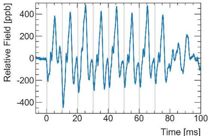
Mechanical vibration of pulsed quad plates drive field perturbations
